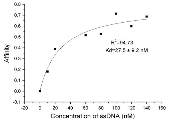
**Fig. 3** Saturation curve and affinity constant (K<sub>d</sub>) of the last pool of enriched aptamers. Affinities were determined using varying concentrations of oligomers and a fixed, excess concentration of inactivated *V. alginolyticus*. Each value represents a single determination. Data were fit to a single binding isotherm
