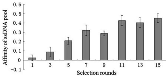
**Fig. 1** Changes in affinity following rounds of selection. Affinity was measured as the absorbance at 450 nm resulting from oxidation of TMB by horseradish peroxidase-conjugated antibody bound to digoxin-tagged aptamers contained within aptamer-target complexes. Results represent the mean of three experiments; *error bars* represent the standard deviation
